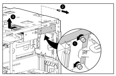
Figure 2-23. Removing the diskette drive
